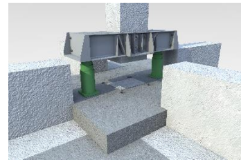
6) insertion of hydraulic jacks, transfer of loads, and cutting of column;
