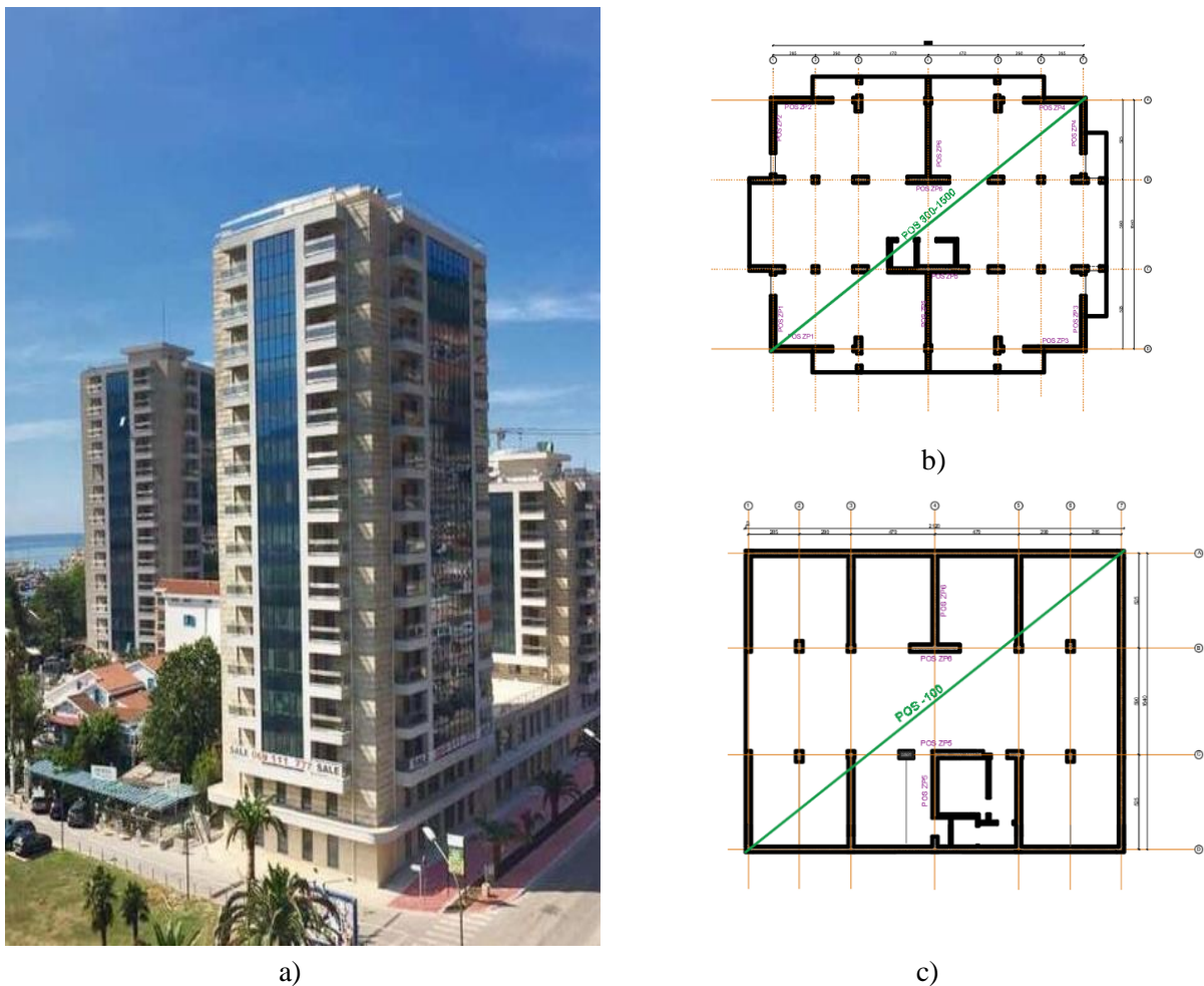
Figure 1. a) existing RC high-rise building; b) floor plan for floors above ground level; c) floor plan for floors below ground level.
