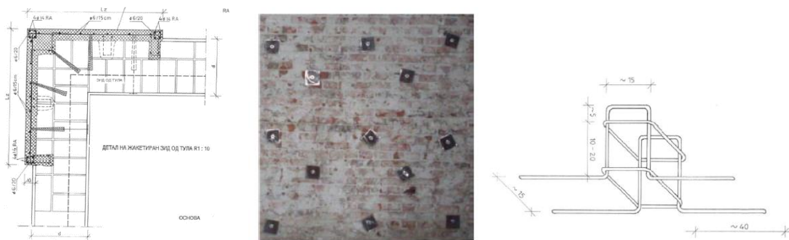
Figure 10. Details of the technology of performance of repair.
