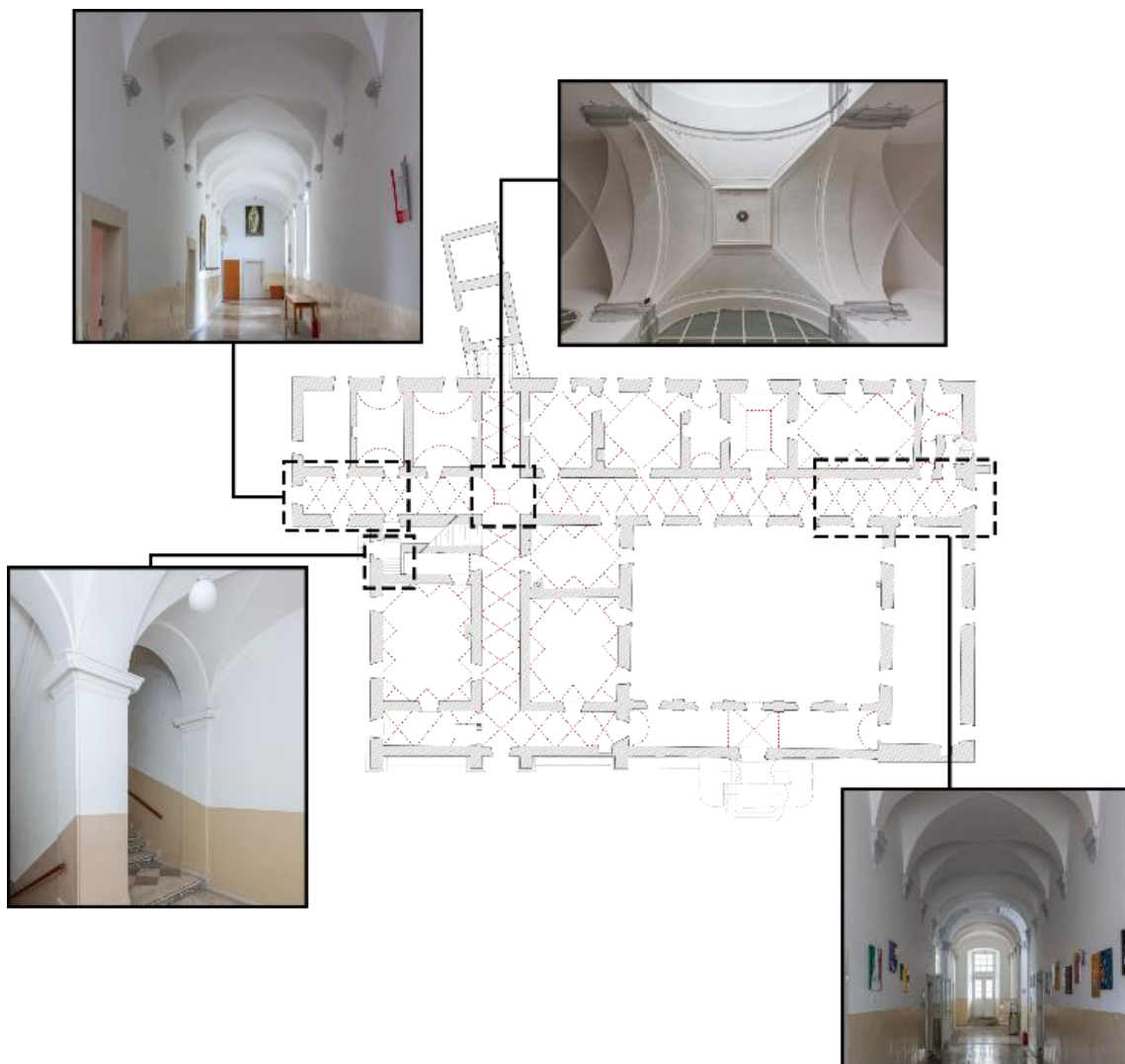
Figure 3. Location and types of different vault systems in the Jesuit College.
