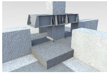
5) insertion of steel structure for upper anchorage of the isolator;
