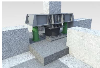
8) loading of non-returnable flat jack & grouting of the isolator's bottom anchorage;
