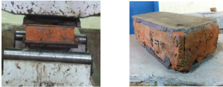
Figure 3 b) Compressive Strength Test of Brick Unit performed at CMTL
