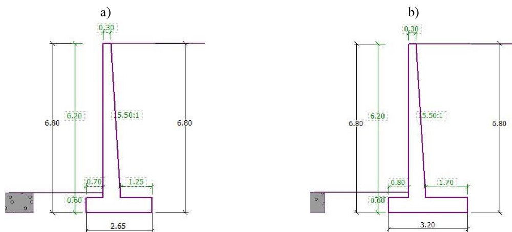
Fig. 2: Obtained foundation width for the wall H=6.0m according to: a) MKS, b) EC 7-1
