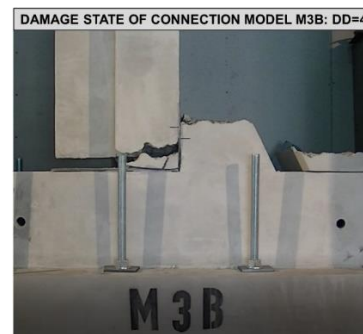
Fig. 14. Damage degree of model M3-B: Typical stage characterized by DD=4.
