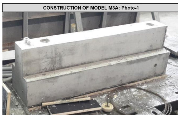
Fig. 3. Construction of model-M3A: Segment of the precast RC floor beam.
