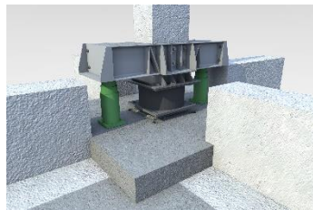
7) insertion of the isolator;
