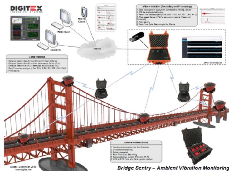
Figure 1. Sentry System Architecture [11].
