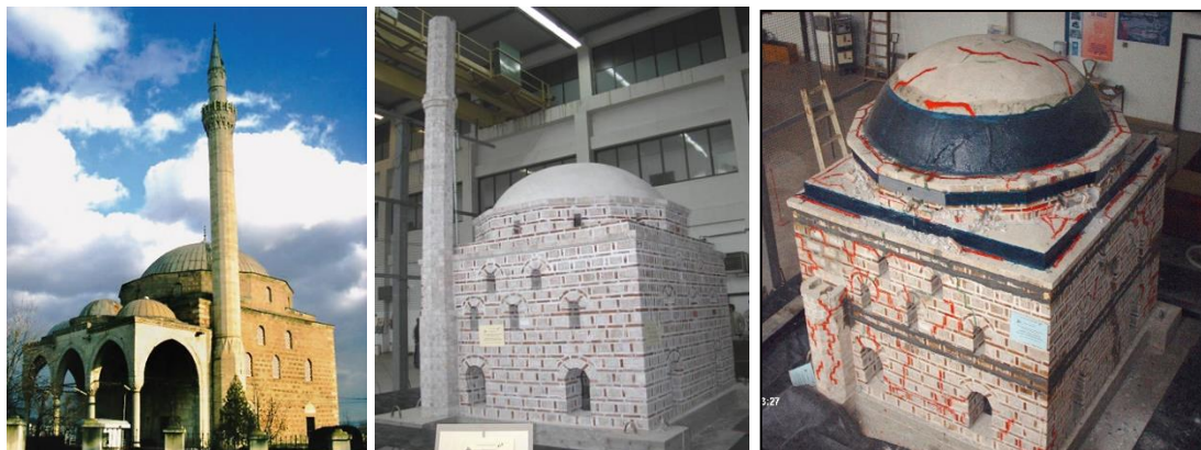
Figure 4. Mustafa Pasha Mosque: prototype (left), 1:6 scaled model (middle), phase 3 – damages (right)
