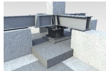
9) removal of hydraulic jacks, installation of beams for the new ground floor;
