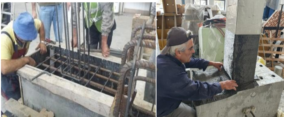
Fig. 2. Construction of the column models for experimental tests and photos taken during application of CFRP on the models.
