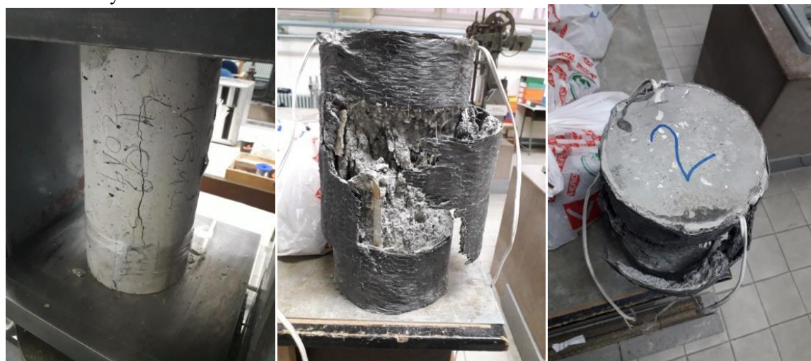
Fig. 6. Testing of the Compressive strength and modulus of elasticity of all three series.
