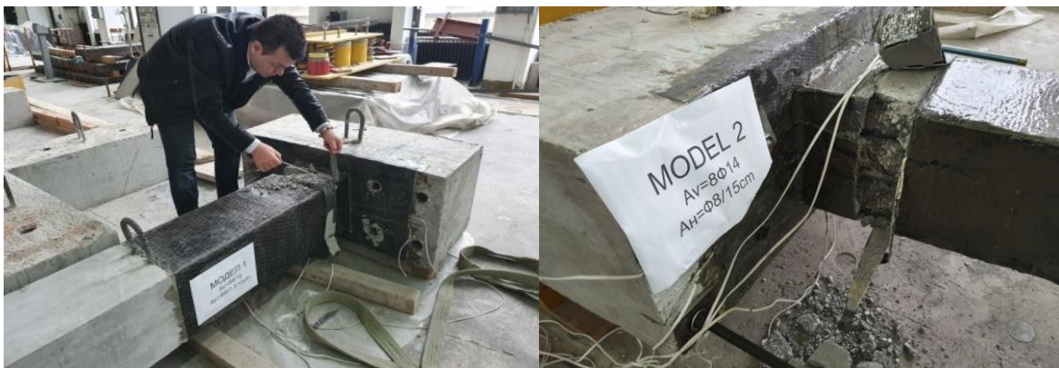
Fig. 5. Observed damages during the quasi static testing of Model M1 and Model M2.
