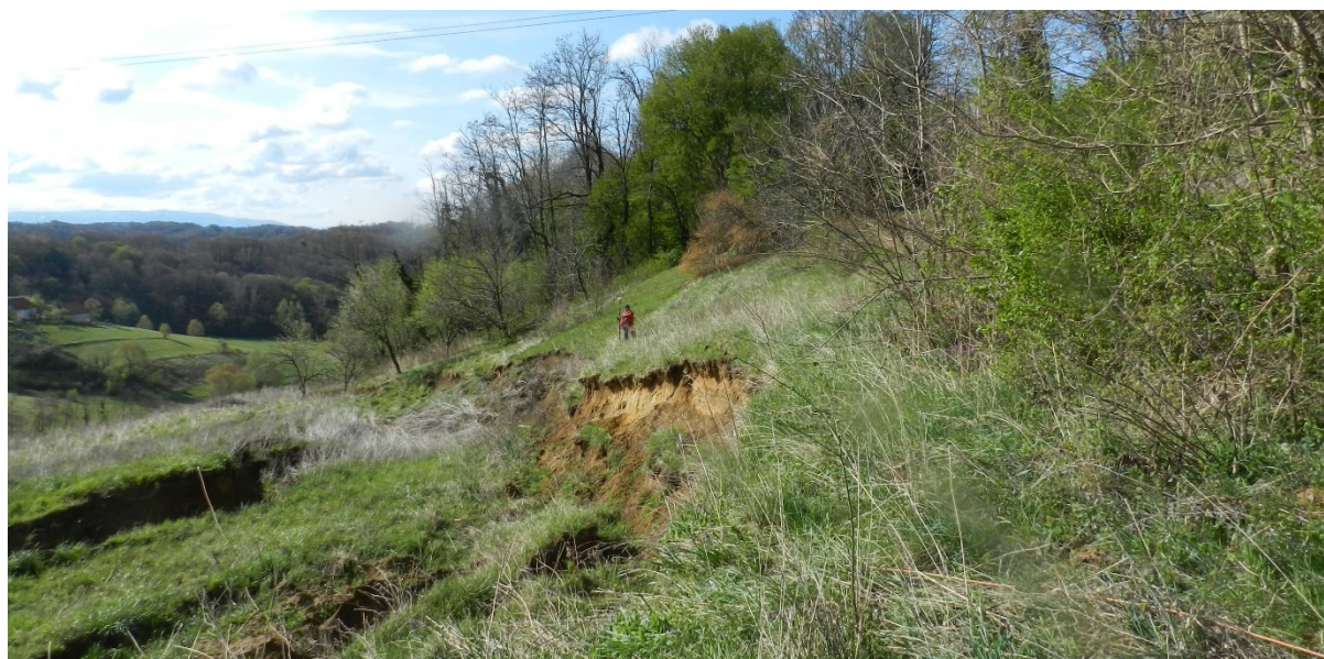
Figure 2. Tensile crack with a jump in the northern part of the landslide.
