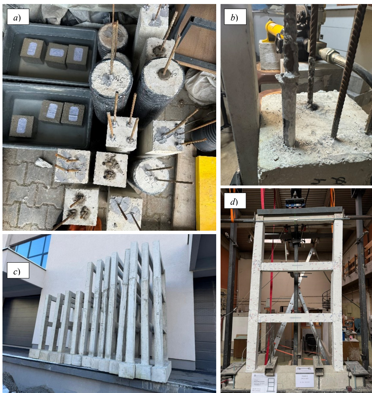
Figure 1. a) Samples for testing different characteristics of the materials; b) pull out of anchors under tensile testing; c) Scaled two- and three-story RC frame models; d) Quasi-static testing one of the frame models.
