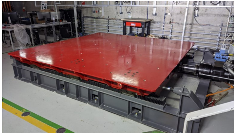
Figure 4: The 1DOF shaking table installed at the University of Minho (PT).
