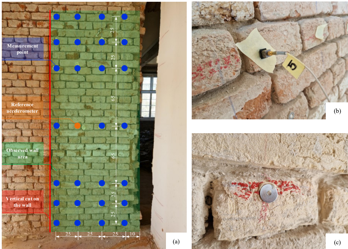
Figure 3. Operational modal analysis set up (a) arrangement of the measurement points (b) accelerometer Brüel & Kjær Type 4508 (c) round metal plate on used during the measurement to place the accelerometers on the wall
