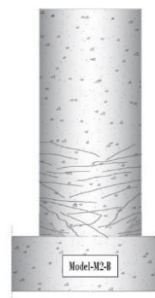
Figure 13. Typical propagation of cracks in concrete during experimental testing of shear failure RC prototype model M2-A.
