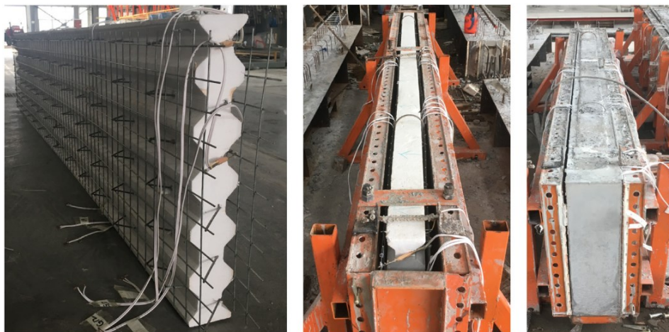
Figure 1. A novel type of sandwich wall panel investigated by Hou, Hetao [16]
