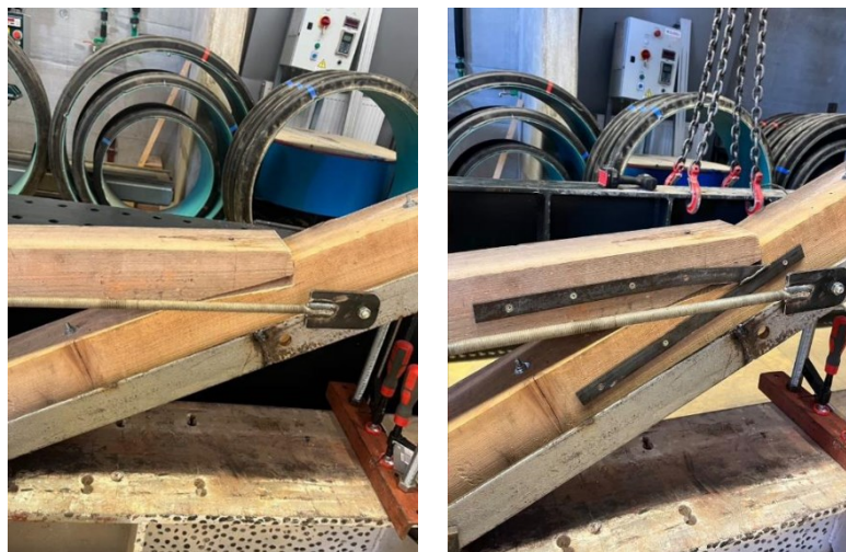
Figure 12. Final deformed shapes of non-strengthened / strengthened joints for 30° skew angle.
