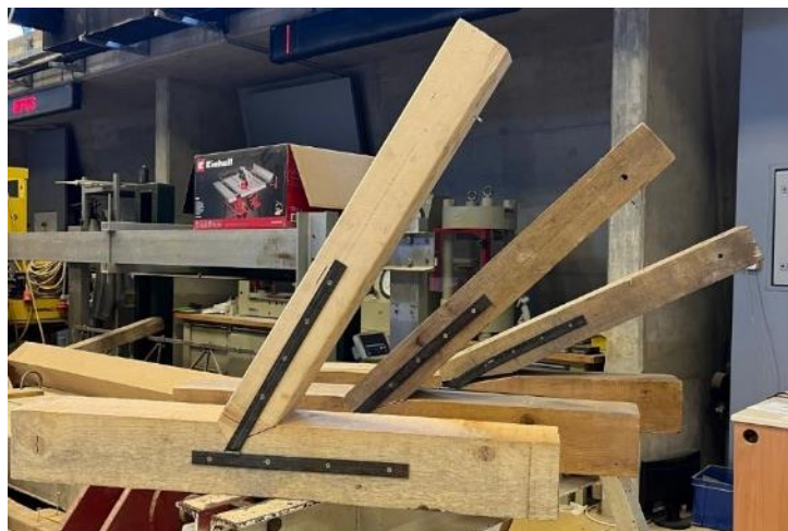
Figure 5. Test specimens of the joint at an angle of 60°, 45° and 30°.
