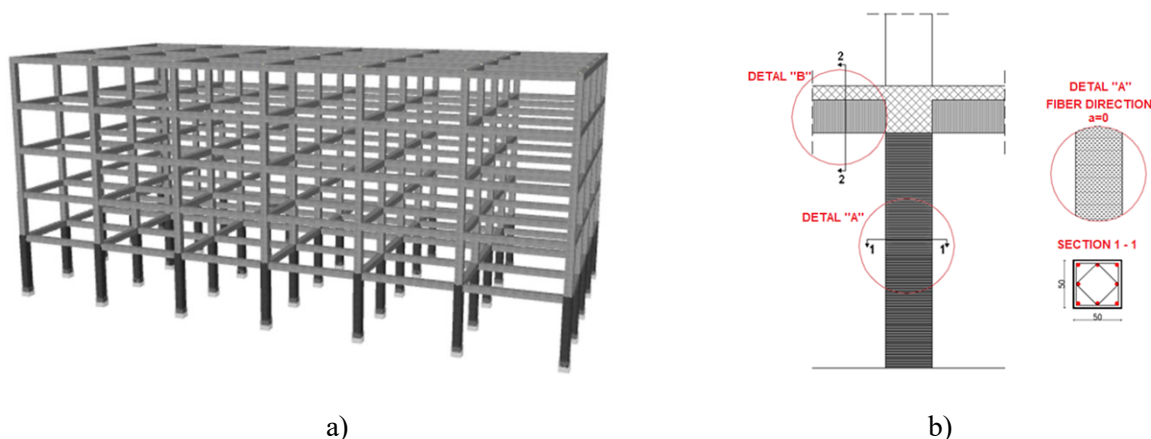
Figure 3. a) 3D model of strengthened structure (Seismostruct computer program), b) Strengthening detail of the columns using CFRP materials
