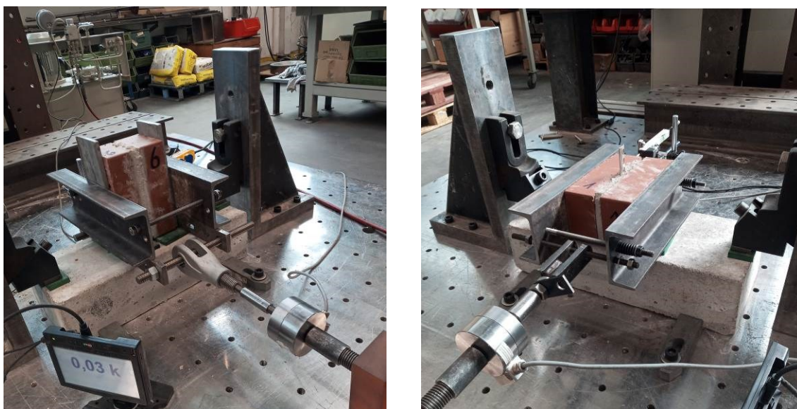
Figure 3. a and b. Test setup for testing the horizontal shear capacity of wall ties in micro scale, a: longitudinal direction of bricks, b: transverse direction of bricks.
