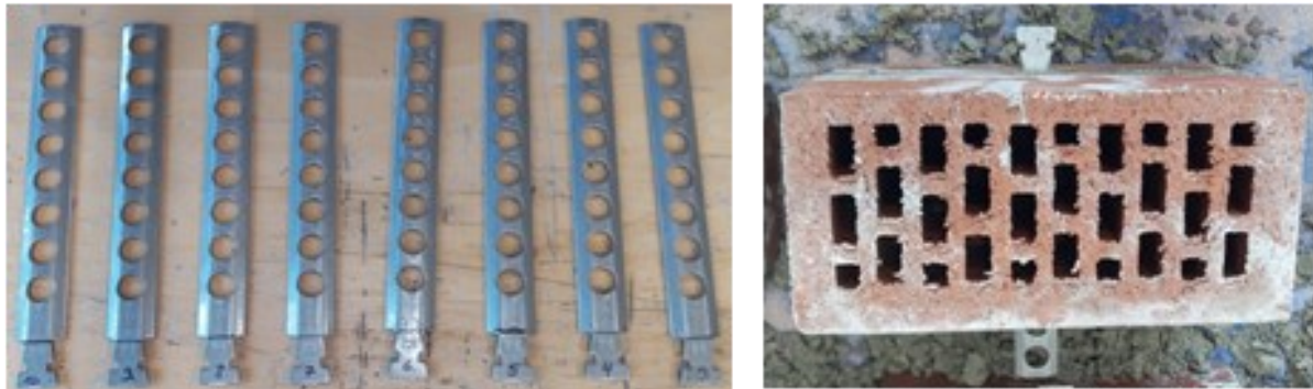
Figure 2. a) tested wall anchors; b) anchors installed in the joint of a brick pair.
