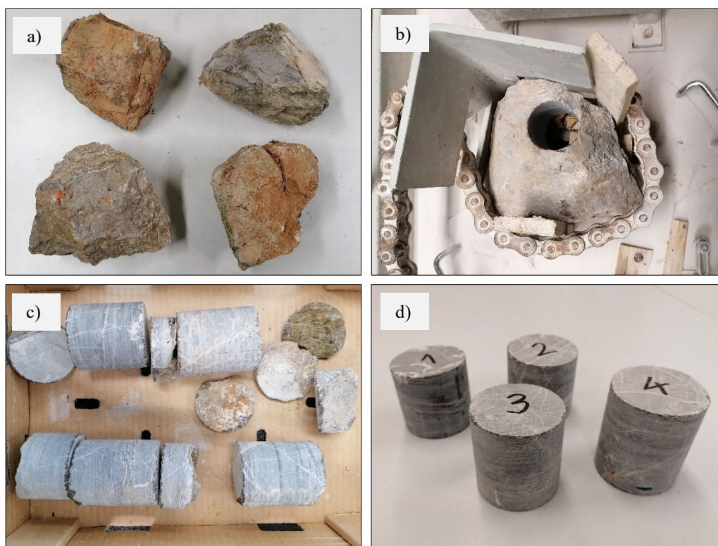
Figure 4. Preparation of stone specimens: a) stone blocks; b) drilling of cylinders; c) extracted stone cylinders; d) specimens ready for testing.
