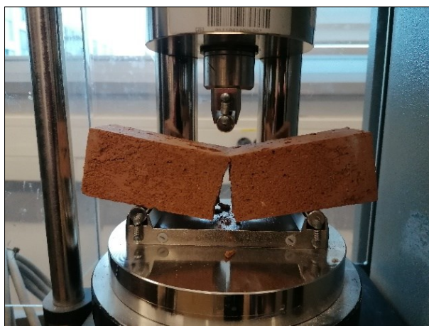
Figure 9. Flexural strength test – three point loading scheme.
