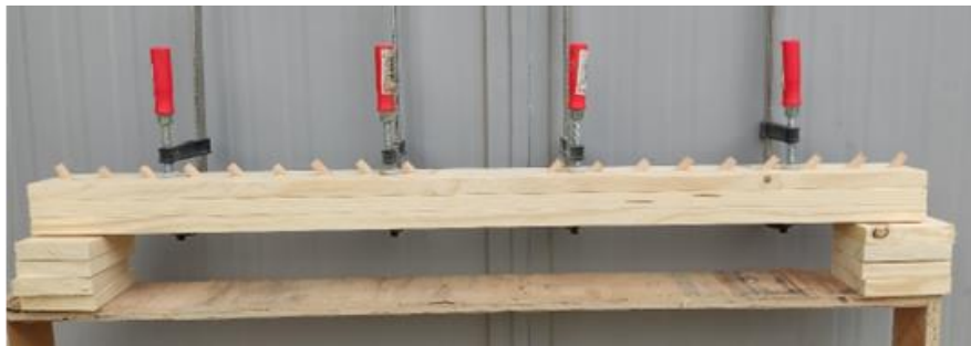
Figure 5. Laminated beam with dowels inserted at 45^\circ (DLT-45)
