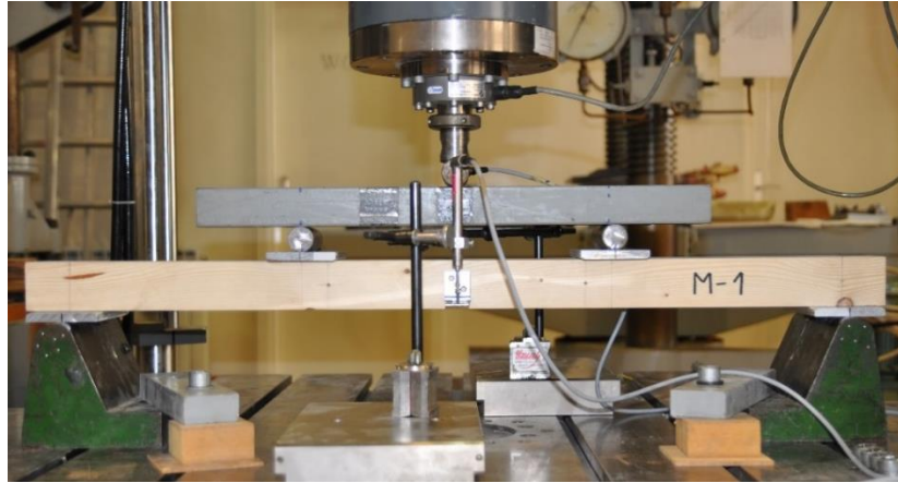
Figure 4. Modulus of elasticity test set-up
