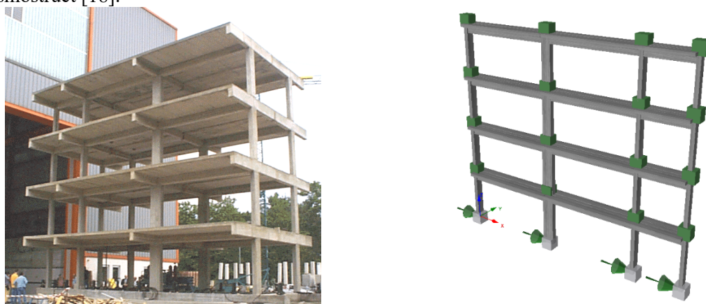
Figure 4. a) ICONS experimental model [17], numerical model of ICONS frame [18]
