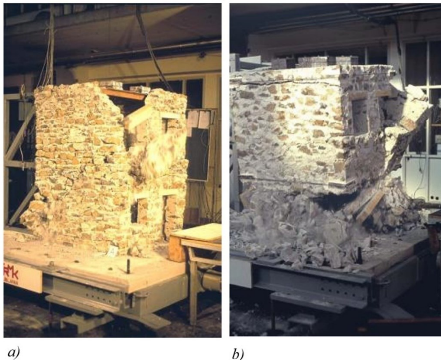
Figure 15. Failure mechanisms obtained by shaking table tests of stone masonry models a) Model without ties; b) Model with wall ties
