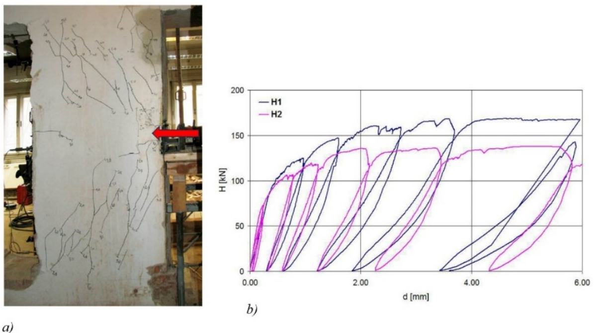
Figure 12. In situ testing of a brick masonry wall. a) Crack pattern after the end of tests. No horizontal cracks at supports can be seen; b) Lateral load-displacement relationships, obtained by monotonic cyclic testing [6]
